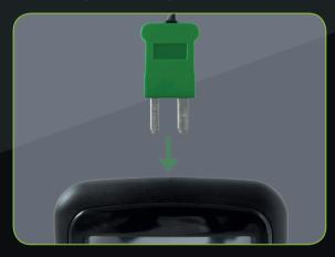
The device is configured to a K type probe. If you wish to use a J, N or T type probe select the settings button and choose the correct probe type.
